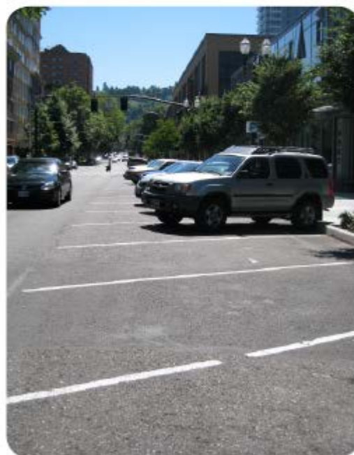
'Back-in' diagonal parking is safer for cyclists than 'head-in' diagonal parking due to drivers' visibility as they exit the parking spot.
